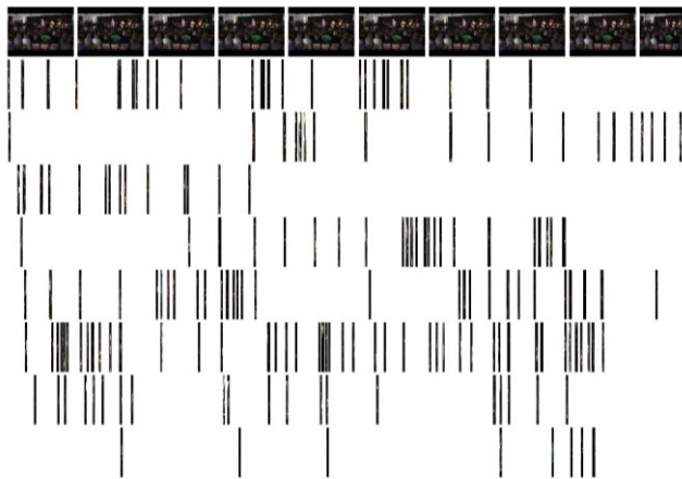
Figure 1 – An example of automatic synchronisation of 187 test signals 5 s each within an event of 1 h 37 min.
