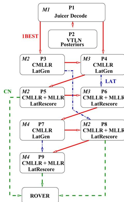
Fig. 6. AMIDA RT'07 system schematic. LatGen denotes lattice generation, LatRescore acoustic rescoring.
