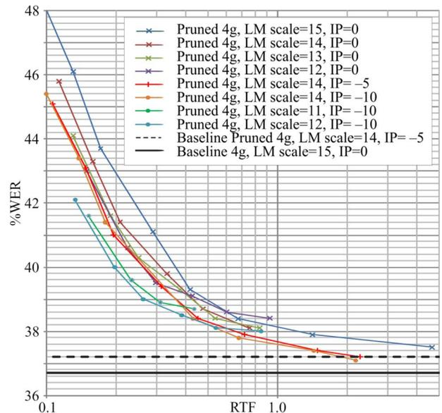
Fig. 5. Real-time factor (RTF) against %WER on *rt07seval* IHM for various decoding arrangements with HTK HDecode and Juicer. “Baseline” refers to lattice generation with a bigram LM and rescored with a 4-gram LM.
