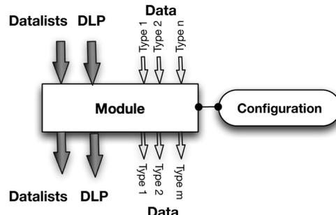
Fig. 7. ROTK modules. Data lists hold metadata such as speaker or segment information, DLP files list data lists and processing information.
