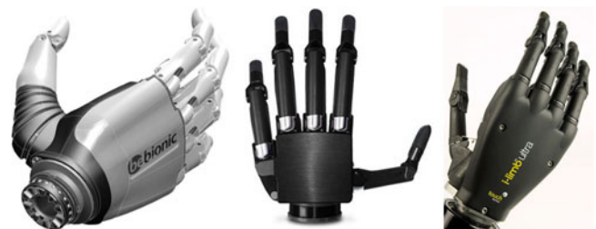
Fig. 1. Dexterous hand prostheses. (From left to right) RSL Steeper's BeBionic (reproduced from www.bebionic.com ), Vincent Systems' Vincent hand ( www.handprothese.de ), and Touch Bionics's i-LIMB Ultra ( www.touchbionics.com ).
