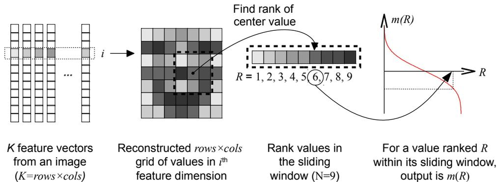
Fig. 2. 2D feature warping for face authentication
