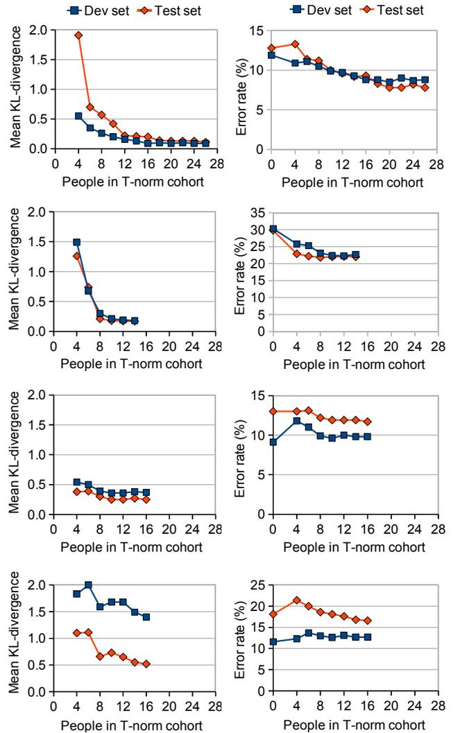
Fig. 6. Results for (top to bottom:) BANCA, SCface, MOBIO (male) and MOBIO (female) databases, showing the effect of reducing the T-norm cohort set size on (left-hand side:) the mean KL-divergence between estimated and actual impostor score distributions and (right-hand side:) the corresponding error rate (% EER on dev set, % HTER on test set) achieved after T-norm is applied.
