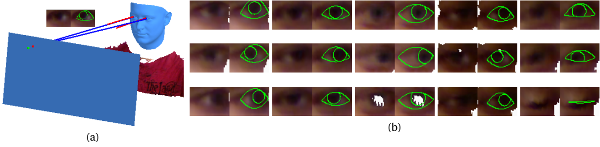
Figure 6.11: Screen gaze estimation task. (a) 3D rendered RGB-D frame. The user’s face region is replaced by the 3D facial template, rendered with the estimated head pose. The blue lines and green dot on the screen are the ground truth. The red lines correspond to the estimated lines of sight and the red dot is the screen intersection (for the left eye). (b) Test images for the left eye (originally, \approx 20 pixels eye width, prior to the pose rectification). The data shown at each column correspond to a different participant. White pixels correspond to missing depth data. The contours represent the mode of q^*(\mathbf{Z}) (the MAP estimate on the geometry).
