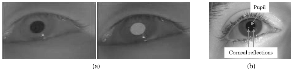
Figure 2.6: IR illumination and sensing for gaze tracking. (a) Dark/bright pupil effect under IR illumination [Hansen and Ji, 2010]. (b) PCCR features: pupil-center and corneal-reflection(s) [Guestrin and Eizenman, 2006].
