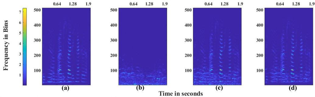
Figure 2: An example of denoising process: Magnitude spectrograms of (a) clean speech, (b) noise signal, (c) noisy speech, and (d) denoised speech. Observe that the denoised speech is similar to the clean one.
