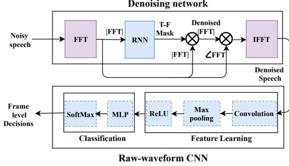
Figure 1: Block schematic of the proposed approach.
