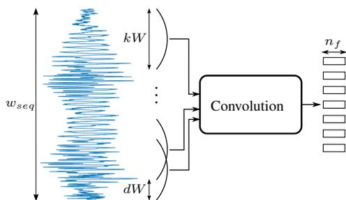
**Fig. 2.** Illustration of first convolution layer processing.
