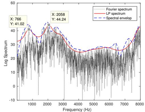
**Fig. 4.** Spectrum of the relevance signal, its LP spectrum and envelop for the speech segment /er/ from CNN3 trained on children speech
