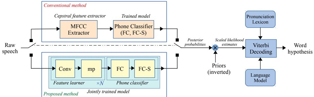
**Fig. 1.** ASR system flow illustrating the conventional and proposed methods. Conv: convolutional layer with ReLU activations, mp: max-pooling layer, FC: fully connected layer with ReLU activations, FC-S: fully connected layer with softmax activation.
