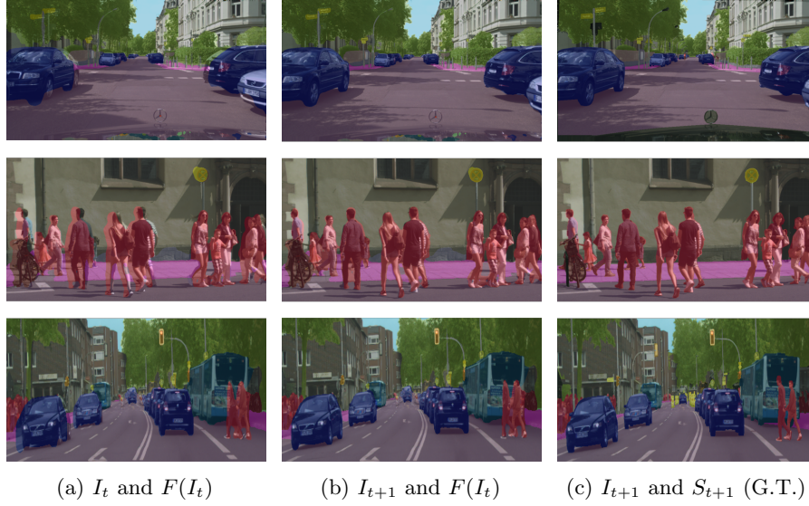
Fig.6: Output segmentation of SwiftNet-R18 trained to predict S_{t+1} from (I_{t-1}, I_t) . We observe a more precise segmentation as the network has a way to infer relative speeds and directions.
