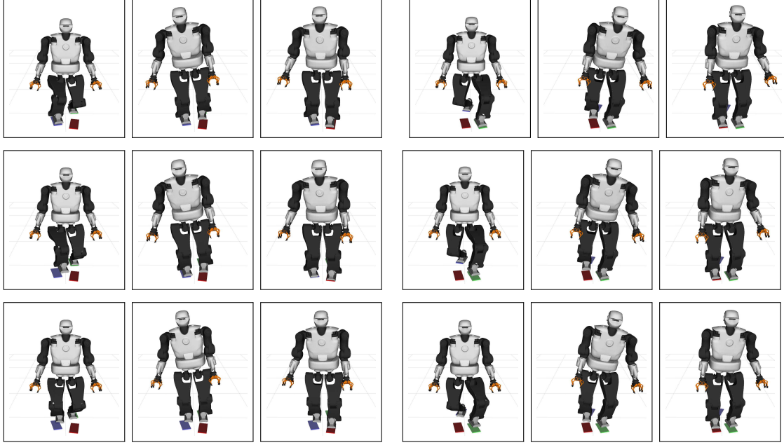
Figure 4.2 – Examples of predicting single-step motions. Warm start produced by Top : GPR, Middle : GMR, and Bottom : k -NN. Left : left foot movement. Right : right foot movement. The green, blue and red box correspond to the initial left, the initial right, and the goal contact pose, respectively.
