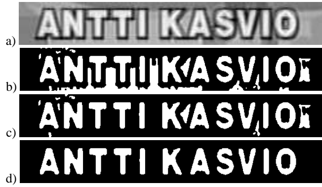
FIG. 7 – Applying grayscale consistency: a) original image b) text layer (3 layers, GBEM algorithm) c) same as b), after the connected component analysis d) same as c), after the gray level consistency step.
