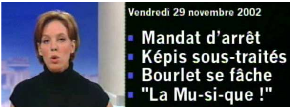
Fig. 10. Examples of video image with compression noise. Despite the large size of text in this image, text distortions are visible (see text).
