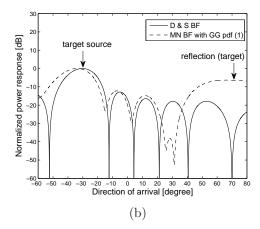
Figure 13: Beam patterns produced by the delay-and-sum beamformer and the MN beamforming algorithm using a spherical wave assumption for (a)  $f_s = 800$  Hz and (b)  $f_s = 1500$  Hz.
