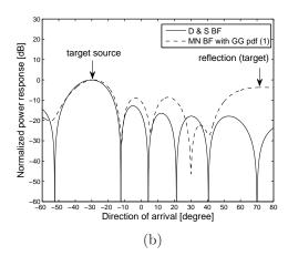
Figure 14: Beam patterns produced by the delay-and-sum beamformer and the MN beamforming algorithm using a plane wave assumption for (a)  $f_s = 800 \text{ Hz}$  and (b)  $f_s = 1500 \text{ Hz}$ .
