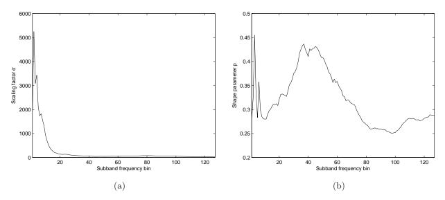
Figure 10: The parameters of the GG pdf for each frequency bin; (a) scaling parameter  $\hat{\sigma}_{|Y|}$  and (b) shape parameter p, where the sampling frequency is 16 kHz.
