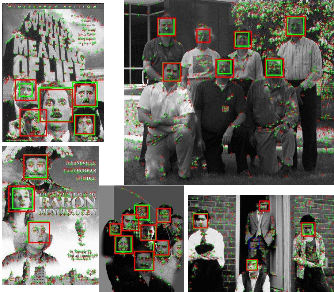
Figure 5.9. Some examples of face detection using interest points on the Cinema and Web face database. The green and red "+" marks represents the interest points detected, the red bounding boxes represent the ground-truth, the green bounding boxes represents the detected faces, and the blue boxes represents false detections.
