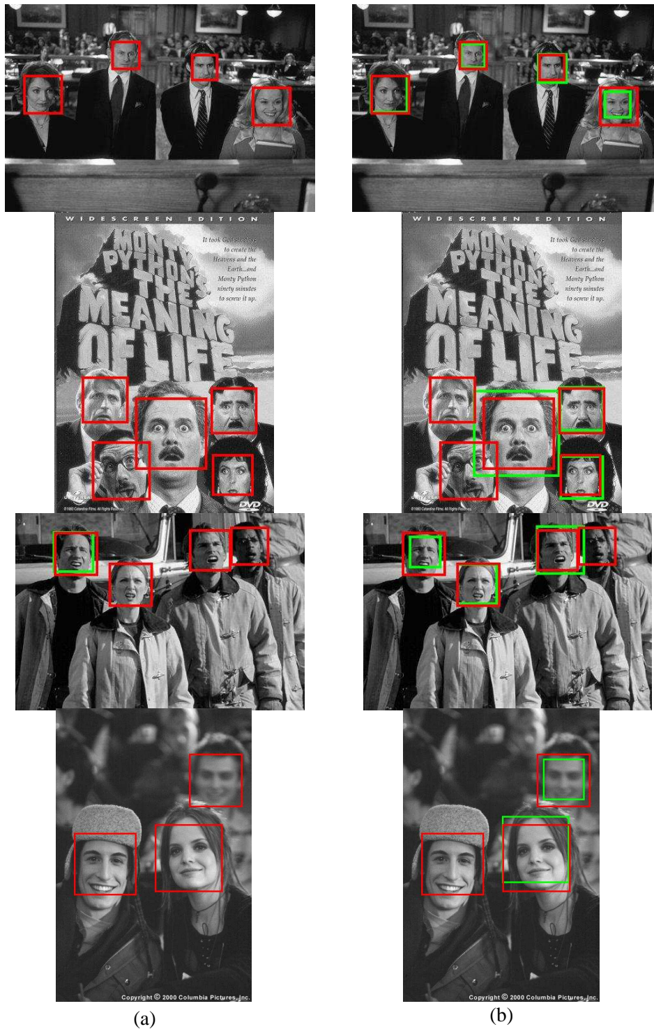
Figure 4.20. Some examples of frontal face detection on the Cinema frontal face database. (a) with standard approach, and (b) with location estimation. The detection results are shown for the scanning grid spacing of 12. The red boxes represents the ground-truth and the green boxes represents detected faces.
