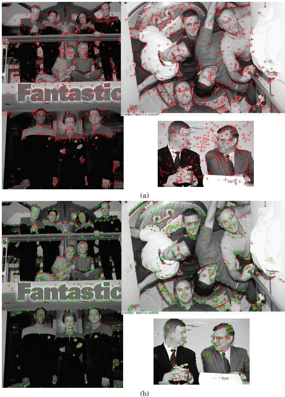
Figure 5.2. Examples of interest point detector on the images containing faces. (a) using difference of Gaussian based detector, (b) our proposed interest point detector based on quantized gradient orientation. The two cross colors represents interest point obtained for two different gradient orientation quantization ( 45^\circ , 135^\circ )(green color) and ( -45^\circ , -135^\circ )(red color).
