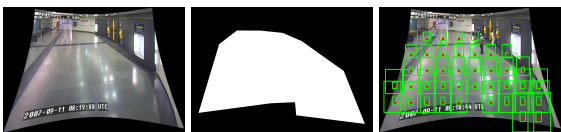
Figure 3: Example of the proposed geometric constraints. Left: scene Middle: binary mask with valid ground plane positions. Right: Sampled ground plane positions (red dots) and valid objects (green bounding boxes). The picture depicts a sparse version of the actual constraints
