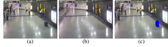
Figure 2: Multi-Layer Static Object Detection (best viewed in color) (a) Original image (b) Layer 1 ( true background ) (c) Generated static object blob from layers L_k > 1 (blue pixels)
