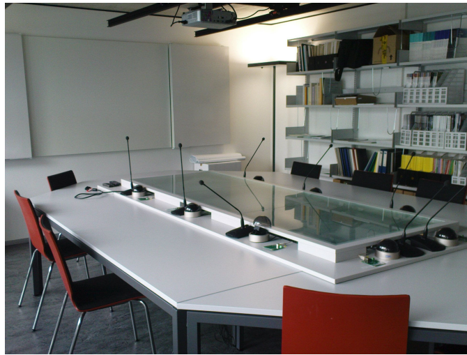
Figure 1.2: Smart meeting room at the University of Fribourg, for up to eight participants (Lalanne et al., 2003). Note the hemispheric casings of the individual cameras and the table-top individual microphones.
