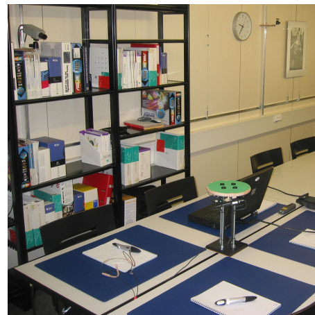
(b) Permanent state of the Idiap SMR. Note the microphone array at the center of the table, with face-capture cameras below it, and a wide-field camera above the books.
