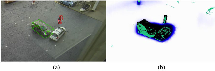
Fig. 4. Simultaneously detecting people and cars. (a) A person and a car is detected, as indicated by the red and green wireframes. (b) The same boxes are projected and filled as black boxes to create a synthetic image that approximates as closely as possible the background subtraction results, shown in green. Note that the white car is the same as the one that appears in Fig. 1. It remains undetected because the background subtraction algorithm fails to extract it.
