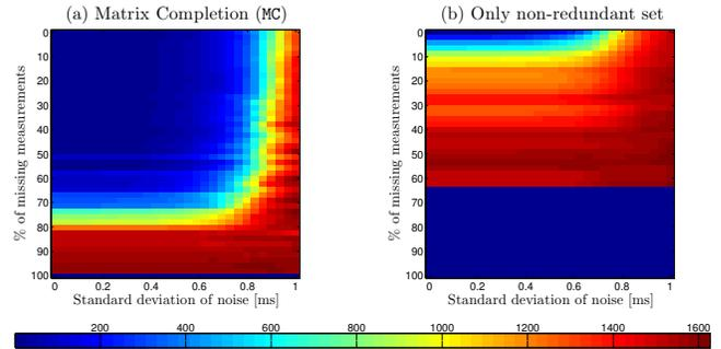
Fig. 4: Missing data recovery in synthetic data: Localization error in mm (using [15], lower is better).
