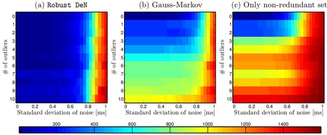
Fig. 2: Robust denoising in synthetic data: Localization error in mm (using [15], lower is better).
