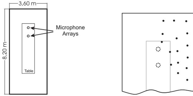
(a) IDIAP room layout showing the centered table, and the microphones arranged in two circular arrays.
