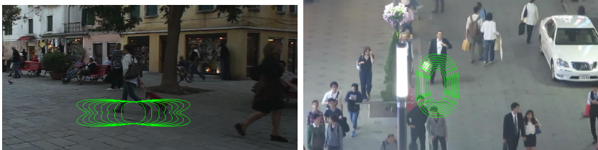
Fig. 2. Position models. The different iso-contours of value 0 of the Potts costs for different values of \Delta (i.e. location of detections occurring after \Delta frames around each shown detection and for which \beta = 0 ), learned from sequences MOT16-01 and MOT16-03. In the region delimited by a curve, association will be favored, whereas outside it will be disfavored. Curves show different moving directions and amplitudes in each sequence.
