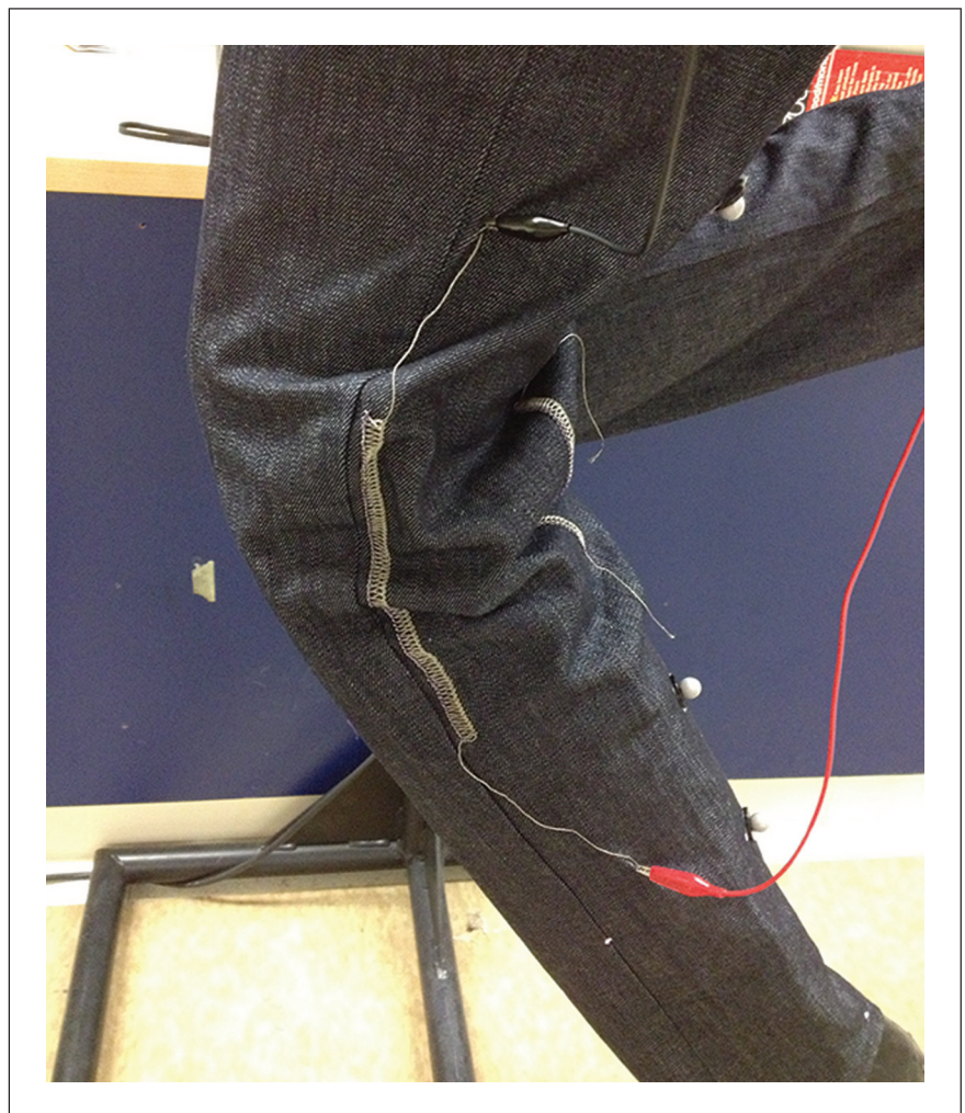
Figure 2. Using conductive fiber to measure a limb angle through the change of resistivity.
