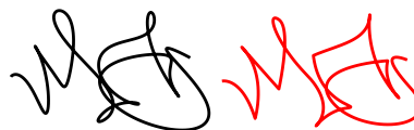
Figure 9: Automatic ligature generation by concatenating the control points of two letters. On the right, a comparative example using Bézier curves.
