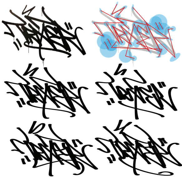
Figure 10: Top left, a graffiti script (tag) made with a marker by Los Angeles artist “Trixter”. Top right, a user defined “motor plan” for the tag, generated by placing targets near salient positions along the original trace and then adjusting the covariances to follow the original trajectory. Second row, the reconstructed trajectory (left) and one variation made by increasing the regularisation parameter r . Bottom row, two random samples from the corresponding trajectory distribution.
