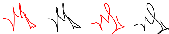
Figure 8: Effect of randomly displacing control point positions with Bézier curves (red) and MPC (black).
