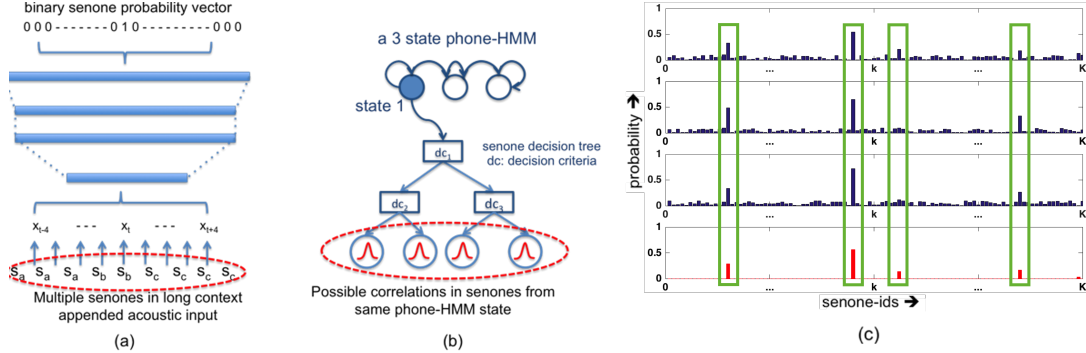
Fig. 1: Correlation among senones due to: (a) long input context and (b) acoustically similar root in decision trees. In (c), we show examples of DNN posterior probabilities for a particular senone class (in blue barplots) which highlight low-dimensional patterns (green boxes) super-imposed with unstructured noise. PCA and sparse coding enable recovery of the underlying patterns by discarding the unstructured noise, and provide more reliable soft targets for DNN training. K denotes the size of DNN outputs which is equal to total number of senones.
