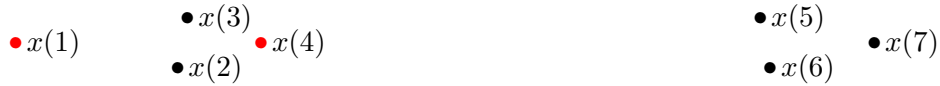
Figure 4.2 – Example with N = 7 samples, of which K = 2 are medoids. Current medoid indices are 1 and 4. Using medlloyd , this is a local minimum, with final clusters \{x(1)\} , and the rest. clarans may consider swap (i_-, i_+) = (4, 7) and so escape to a lower MSE. The key to swap-based algorithms is that cluster assignments are never frozen. Specifically, when considering the swap of x(4) and x(7) , clarans assigns x(2) , x(3) and x(4) to the cluster of x(1) before computing the new MSE.
