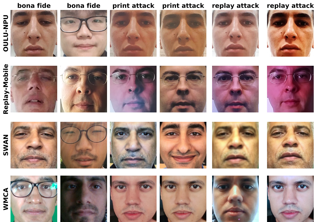
Figure 2.15 – Examples of domain shift between datasets in face PAD. The samples of each row belong to the same dataset. The datasets from top to bottom are OULU-NPU, Replay-Mobile, SWAN, and WMCA. The first two columns are bona fide samples, the second two columns are print attacks, and the last two columns are replay attacks. Samples from each class can change drastically between datasets. The identity of the person, pose, illumination, camera device, PAI used to create the attack, and other factors are the cause of domain shift between these datasets.
