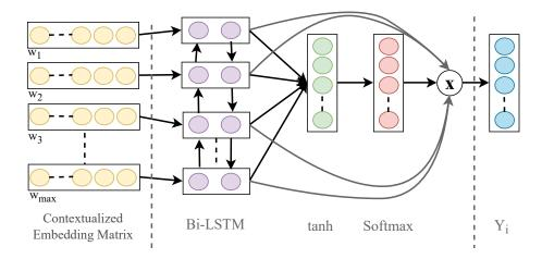
Figure 2: Architectural illustration of the attention mechanism used in the proposed model
