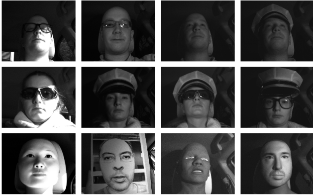
Figure 4. Samples of presentations from VFPAD dataset demonstrating variations in accessories, pose, and illumination, etc. The upper two rows consist of bona-fide samples, and the bottom row depicts presentation attacks. The images, captured in 12 bit resolution, have been converted to 8-bit representation by discarding lower 4-bits.
