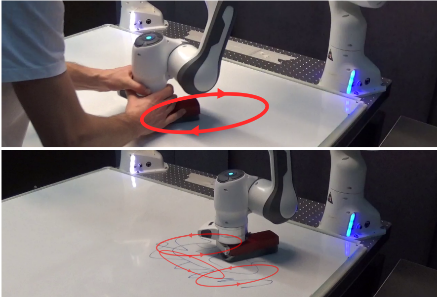
Figure 3.1 – Rhythmic tasks such as wiping need to be demonstrated in few demonstrations ( top ), while the robot should extract the important motion features (e.g. amplitude, frequency and phase) and generalize it in a consistent, safe manner ( bottom ).
