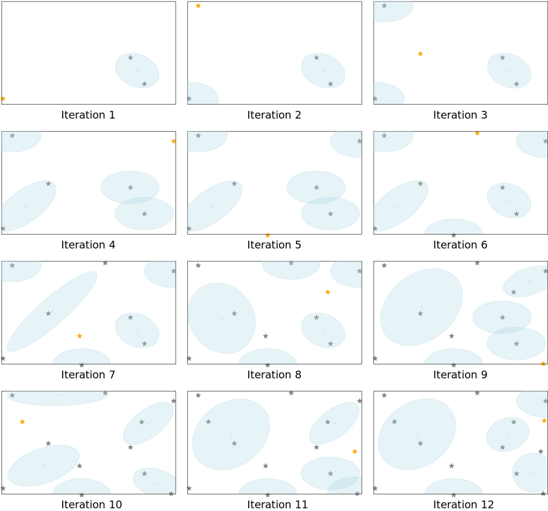
Figure 5.3 – Evolution of the active imitation learning strategy. The goal space is represented in this figure. Grey stars represent the final object position of the available demonstrations, and orange stars the selected goal to query. The transparent ellipses show the marginal distribution of the BGMM on the goal space.
