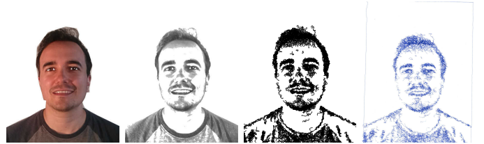
Fig. 3: Intermediary outputs of the processing pipeline. From left to right: Original image taken by the robot. Processed image that is used as input to the coverage algorithm (inverted). Strokes that were computed using the coverage algorithm. Final portrait drawn by the robot.
