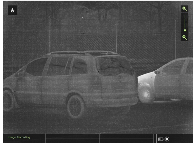
Figure 6. Illustration of ill-posedness of the image-to-image translation problem for visible to thermal conversion. The two images (thermal on the left, visible on the right) were taken at around 9am at an outside temperature of 6°C. The car on the left had remained parked overnight while the car on the right had just recently been used.
