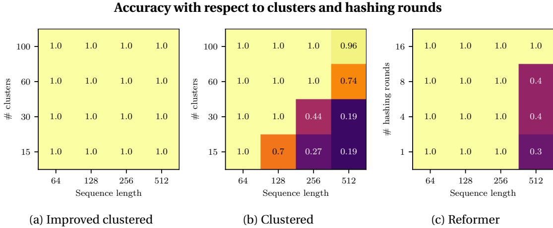
Figure B.3: The heatmaps depict the achieved accuracy on an artificial copy task (Appendix B.3.1) as the sequence length, the number of clusters and the number of hashing rounds varies. Improved clustered (Figure B.3a) is the only fast transformer variant that can solve the task perfectly for any sequence length and number of clusters combination.
