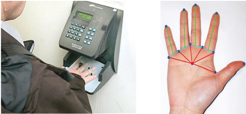
Figure 17: Palm geometry device and some palm features.
