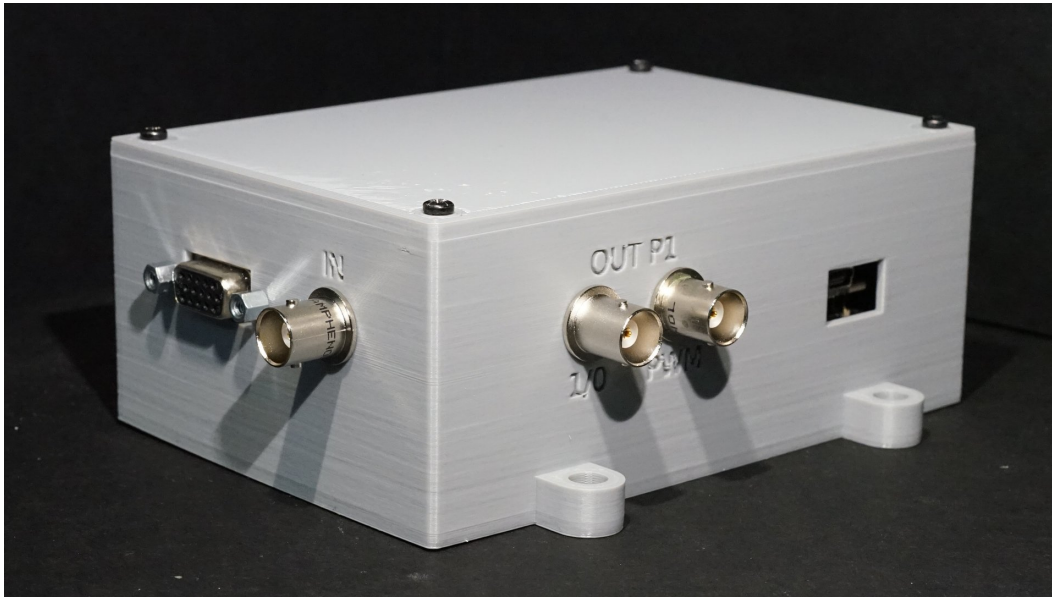
Figure 1.3: The controller in its 3D-printed protective case. Standard BNC connectors allow maximal compatibility with most imaging hardware.
