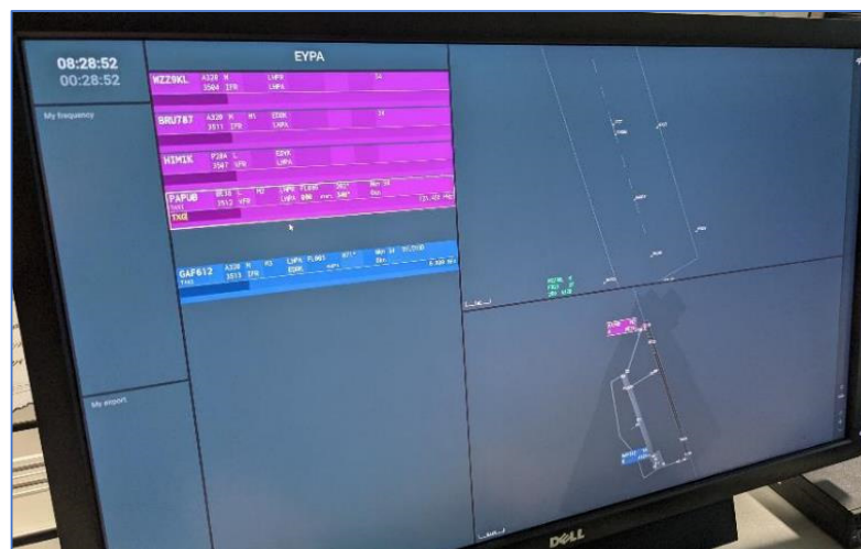
Figure A3. Simulation pilot interface for a simulated airport with time, pseudo flight strips for arrival and departure traffic, and radar views for airport surface and surrounding.
