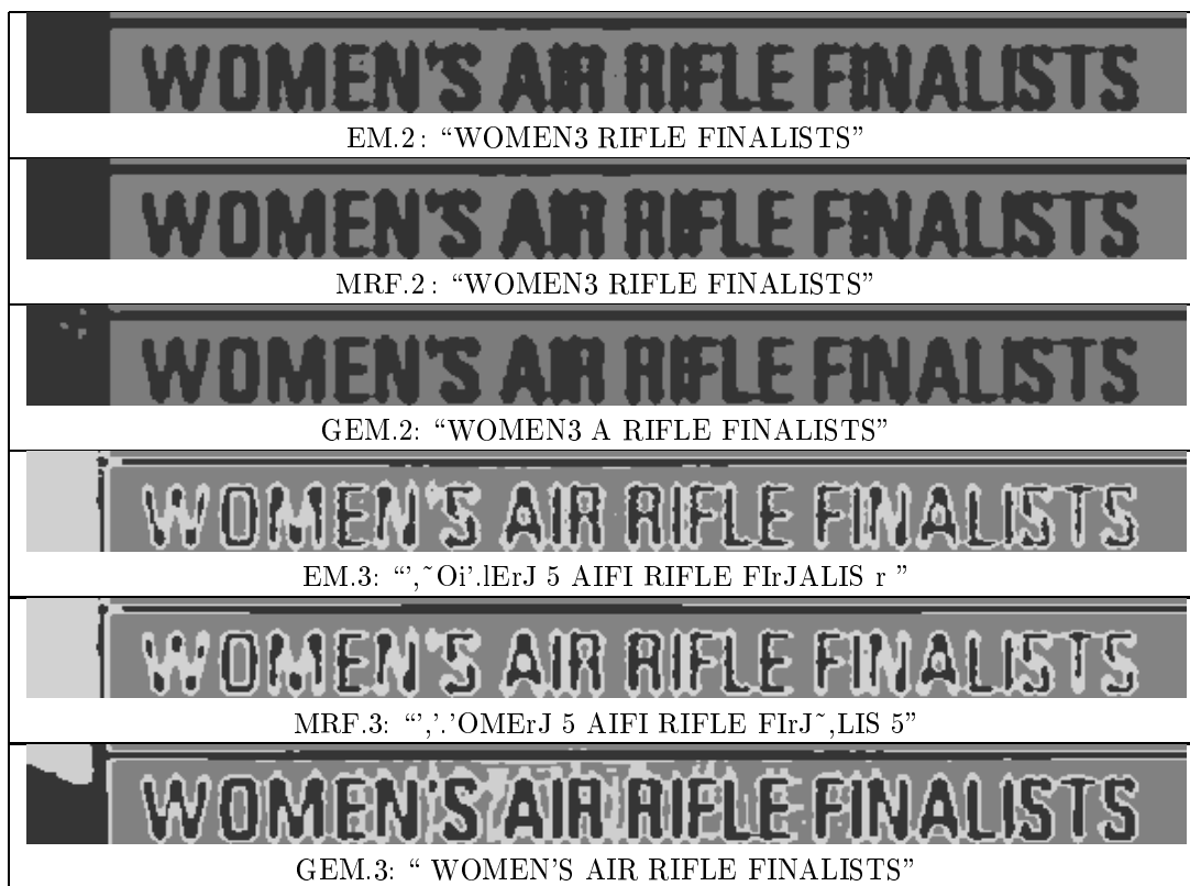
FIG. 3 – Noise adaptive: Segmentation output of the present 3 algorithms and recognition results using 2 and 3 Gaussians.
