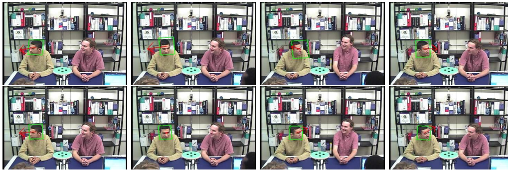
Figure 6: Sample of tracking failure for MSPF due low number of samples. First row : MSPF; Second row RBPF.
