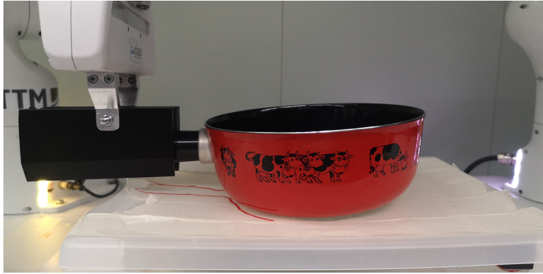
Figure 4.14: Test with the 3D printed left gripper, it can correctly grasp and lift the bowl.
