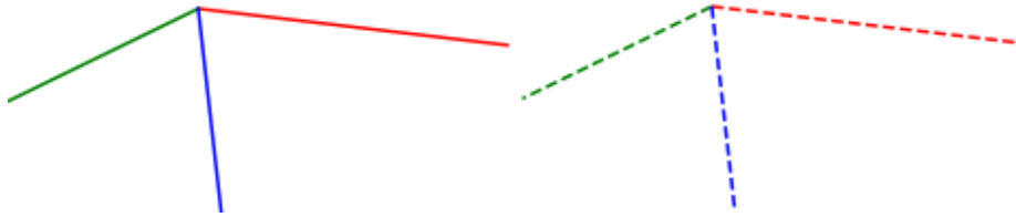
Figure 4.5: The left image represents the desired final orientation of the end-effector frame, and right image represents the planning solution to the final orientation of the end-effector frame. As you can see, these two orientations are the same. This is a visual test to see if the planning worked as expected.
