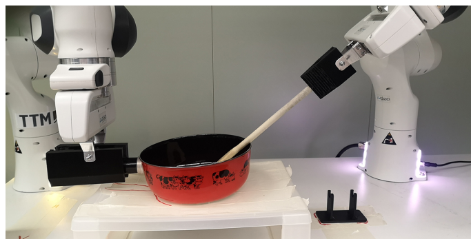
Figure 4.17: Test with the 3D printed right gripper, where it grasps the spatula. In this picture, you can also see the left robot maintaining the fondue bowl.
