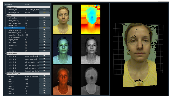
Fig. 6. Interface developed for visualizing the alignment procedure. The best calibration and parameter tuning can be selected based on this tool. On the right side of the interface, any channel (here RGB) can be projected in 3D and then after rectification reprojected to get same alignment between all channels.
