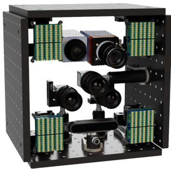
Fig. 3. Sensor suite used for the data collection in HQ-WMCA dataset.
