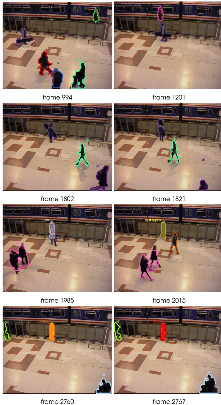
Figure 8.13. Abandoned luggage item detection results. Video results for detecting left luggage items for sequence S5 from the PETS 2006 data corpus. The luggage owner is seen arriving in frame 994, loiters for a bit (frame 1201), and places his snowboard against the wall between frames 1802 and 1821. In frame 1985 the bag is detected, but the owner is still within the attending limits. In frame 2015, the model has determined the owner is more than 3 meters away from the bag, and marks the bag as unattended . In frame 2760, 30s have passed since the owner left the 2 meter limit, and a warning is triggered (ground truth warning occurs in frame 2749). In frame 2767, 30s have passed since the owner left the 3 meter limit, and an alarm is triggered (ground truth alarm occurs in frame 2764).
