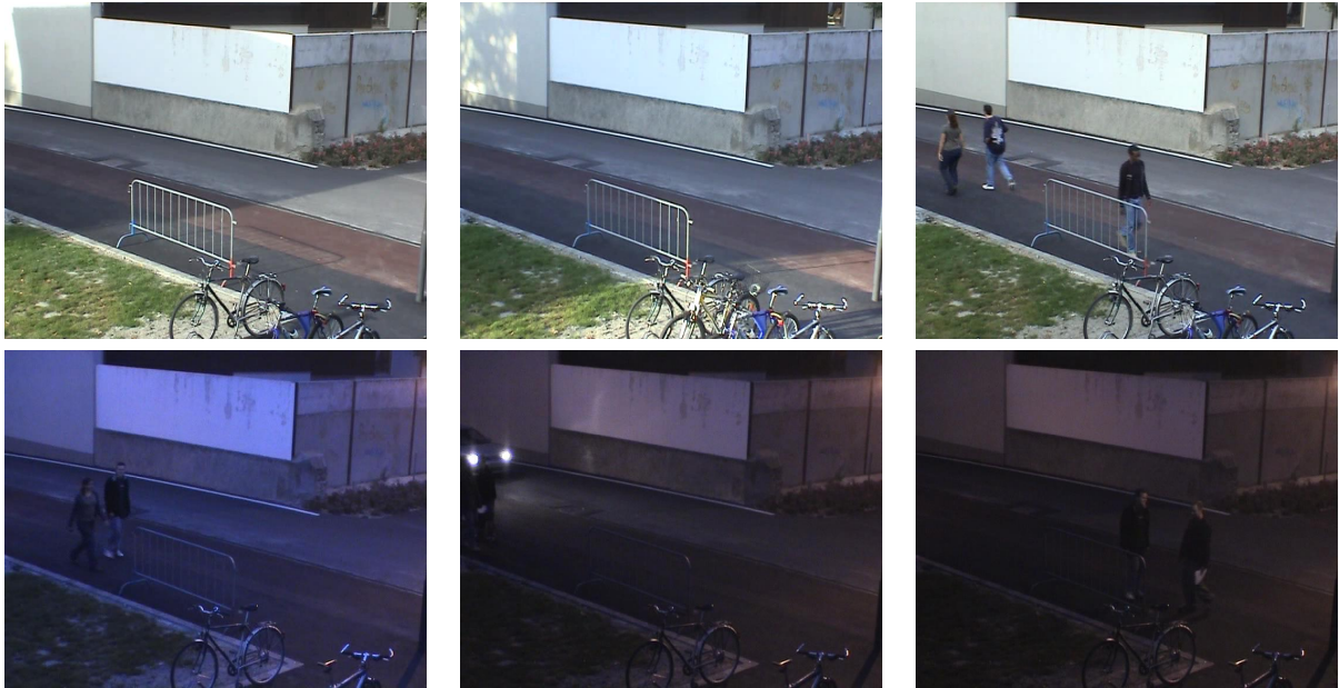
Figure 2.4. Appearance changes resulting from changes in illumination. The six images above were extracted from a video recorded over the course of only three hours. The effects of shadows and changing illumination sources on the appearance of objects in the scene is dramatic. Such appearance changes pose a problem for object modeling in tracking methods.
