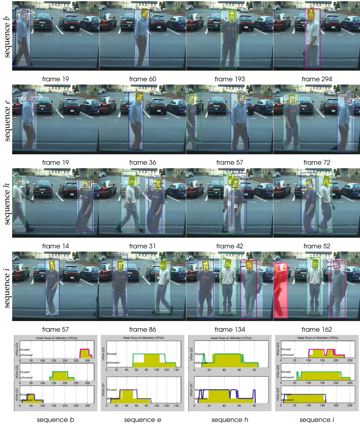
Figure 7.12. Tracking and WVFOA results. Results for four sequences, b , e , h , and i . A summary plot of the WVFOA performance is provided at the bottom. For details on interpreting the plots and symbols, refer to Fig 7.8. Here, we can see the WVFOA performance was nearly perfect for sequence b and exhibited slight errors in sequence i . The 2 nd person (green) in sequence e suffered from prematurely estimating a focused state. Sequence h suffered some ambiguities due to the loss of head tracking as people crossed paths. Frame 162 of sequence i shows a FP error generated as a tracker was placed where no ground truth was present. Though the subject is half-visible as he exits the scene, no ground truth was annotated. This demonstrates the ambiguous problem of defining exactly when a person appears in the scene.
