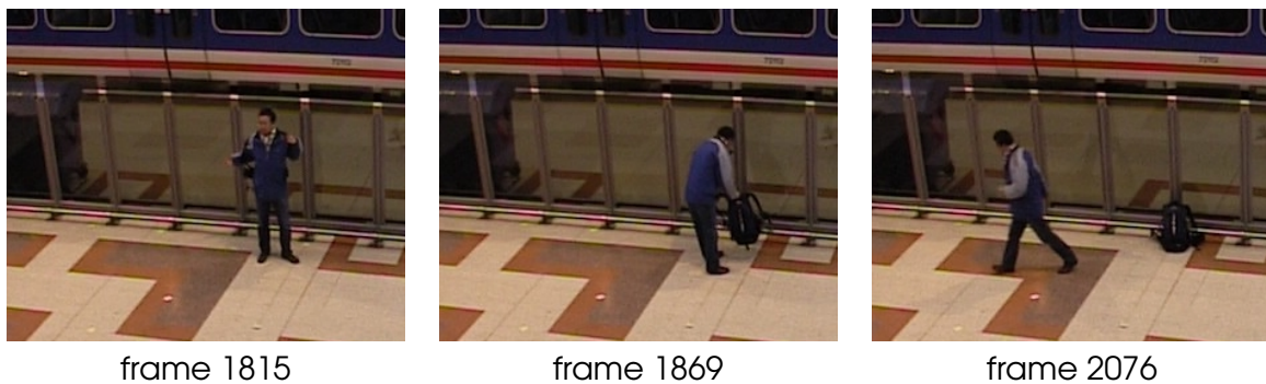
Figure 2.2. An activity recognition task. Human activity recognition attempts to recognize discrete activities which often occur over a limited time duration. An example of a human activity recognition task is to determine when a luggage item has been left unattended. In the images above, a man sets his backpack on the ground and walks away.
