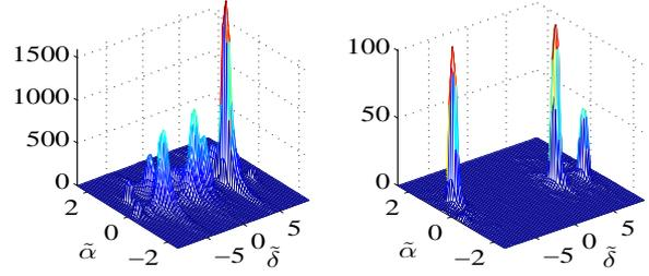
Figure 1: Left: Fullband weighted histogram, Right: Subband weighted histogram ( $100 \leq \omega \leq 570$ ). The actual number of sources is 3,  $p=0.5$  and  $q=1$ . Distance between microphones is 0.03m.
