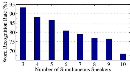
Figure 3: Spectro-temporal disjointness of overlapping speech quantified in terms of ASR performance
