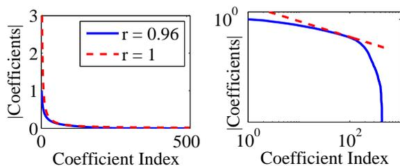
Figure 4: Power-law decay of the recovered t-f components depicted in linear (left) and logarithmic (right) axes.
