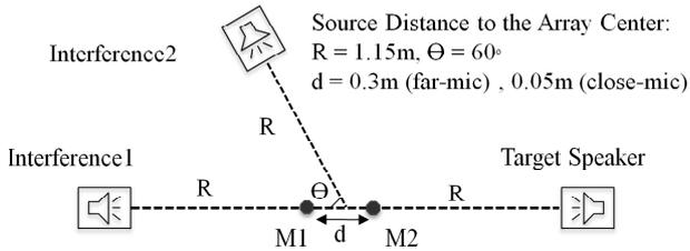
Figure 2: Overhead view of the room set-up
