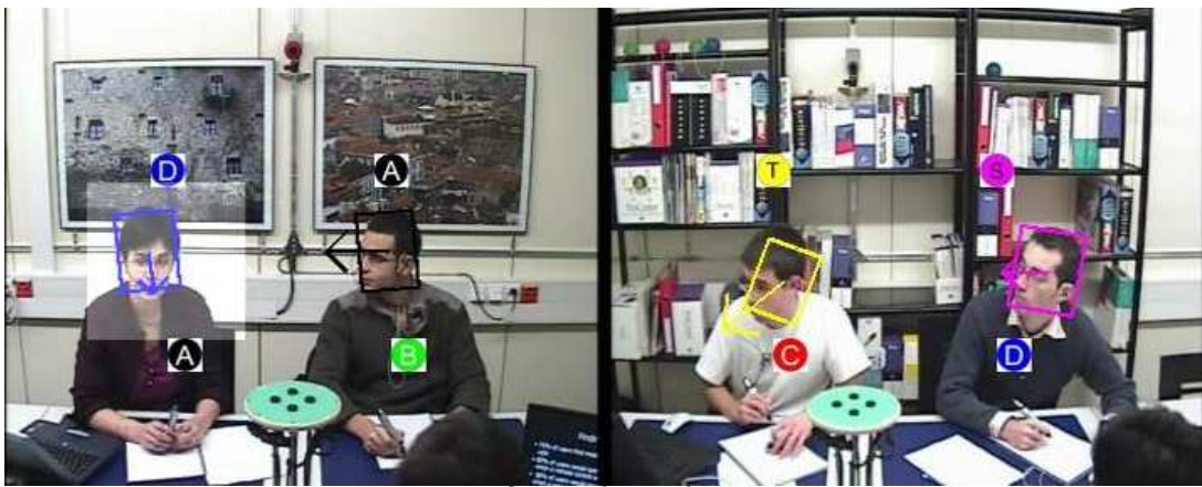
Figure 2.5. (a). Shows the top view of the meeting room. (b). Shows the side camera views and the estimated visual focus of participants using side-view camera views. Each of the participants is labeled and their focus of attention is displayed above their head (T stands for Table and S stands for Slide-screen). Colored rectangle around the head shows the head location and colored arrows shows the head pose of each of the participants. The white transparent box placed on participant A shows that her speaking status is 'true'.
