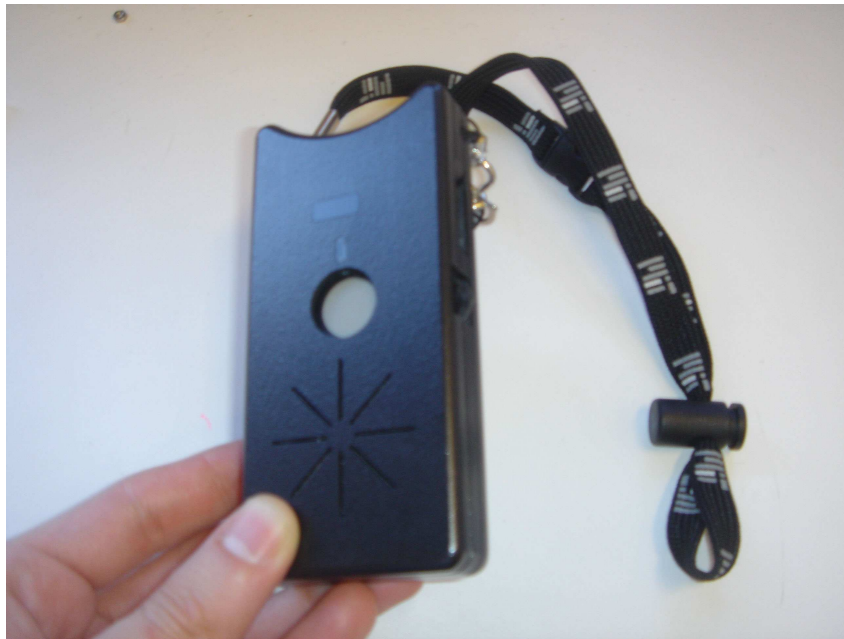
Figure 4.7. Sociometric badge developed by Human Dynamics group, MIT Media Lab (Olguín and Pentland, 2008).
