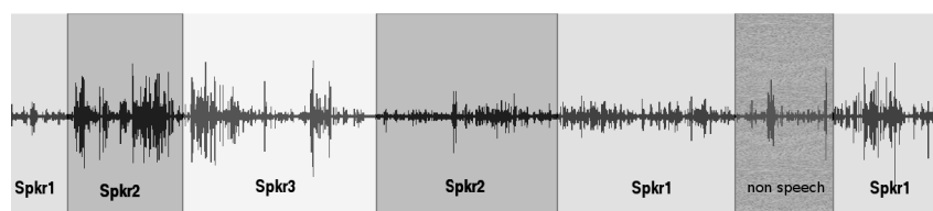
Figure 2.1. Speaker diarization consists of detecting number of speakers and speech corresponding to each speaker
