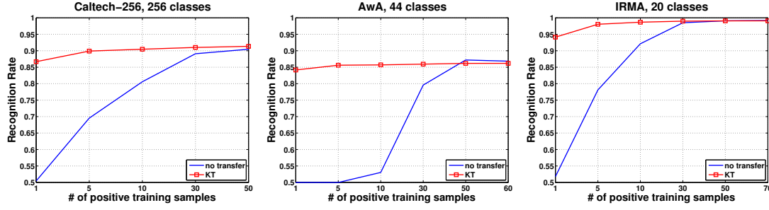
Figure 3.10 – Recognition rate as a function of the number of positive training samples. Each experiment is defined by considering in turn one of the classes as target and the others as sources and extracting randomly the training samples ten times. The final results are obtained as average over all these runs. The title of each plot indicate which dataset have been used.
