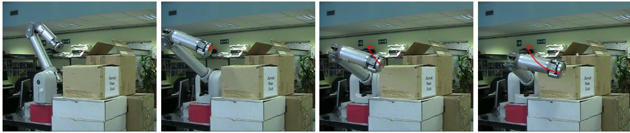
Fig. 4. Execution of the task on the WAM arm. The red line represents the trajectory of the end-effector.
