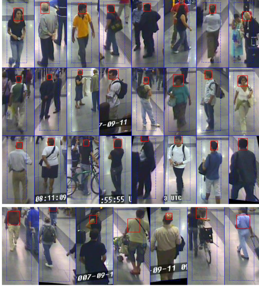
Figure 6.3: Head localization results. Dashed blue boxes are the human detection outputs. Solid red boxes are the head localization outputs (first candidate for each bounding box). Failure cases are shown in the last row.
