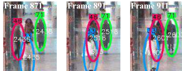
Figure 5.14: Identity switch example on CAVIAR. Person with id #46 comes out of a shop then gets occluded in the next frames. Another person that was previously occluded takes his label. Images were zoomed in around the location where the IDS takes place.
