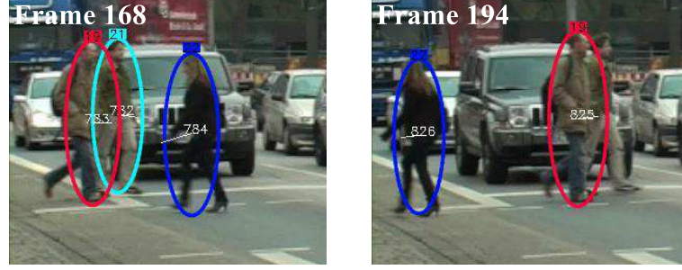
Figure 5.6: Effect of missed detections near the end of the sequence on TUD-Crossing. A person is detected for the last time in frame 168 and is assigned label #21. The person is not re-detected before the end of the video. As we do not propagate detections nor extrapolate tracklets, tracking is lost for that person. Images were cropped to highlight the misdetection.
