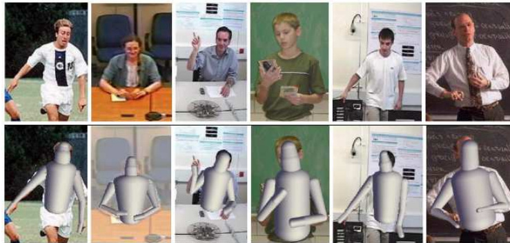
Figure 2.11: Sample upper-body pose estimation results obtained by [Lee and Cohen, 2004]: original images (top), estimated pose (bottom).
