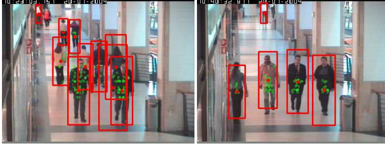
Figure 2.3: Examples of detector outputs showing (left) a missed detection and a false alarm; (right) detection accuracy issues, like legs cut or extended due to projected shadows on the floor. Detections were obtained with the code of [Yao and Odobez, 2008a] 2 .
