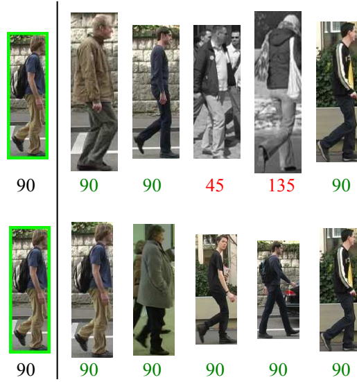
Figure 6.15: Illustration of KNN for the same query image (highlighted) in original feature space (first row, 2 mistakes) and in the biased manifold (second row, neighbors have the same pose).
