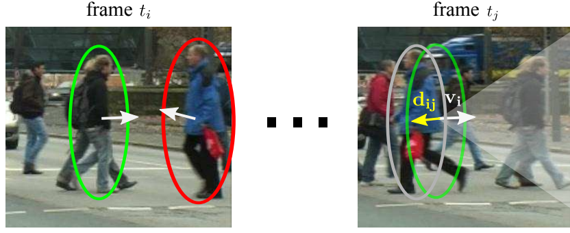
Figure 3.4: Role of the visual motion for tracking. Left: detection r_i at time t_i along with its estimated visual motion \mathbf{v}_i (green ellipse). Right: in subsequent frames, the motion cost associated to this detection at t_i favors associations with other detections located in the direction of motion (shaded area) and penalizes associations in opposite directions (example of blue person, gray ellipse).
