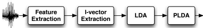
Figure 3: I-vector system using PLDA scoring. The LDA and PLDA modules are trained to discriminate labels defined by the task, i.e. speaker, accent or language labels.
