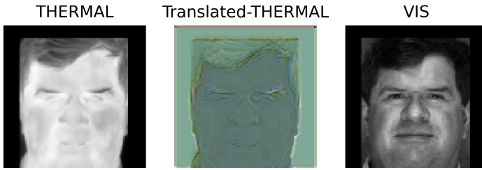
Fig. 6 An illustration of thermal to vis HFR scenario in Polathermal dataset, the Translated-Thermal is the intermediate output from the PDT module. Although this 'Translated-Thermal' image may not visually resemble the VIS image, the embeddings generated from it align closely with those from the VIS image, as indicated by the high matching scores achieved.
