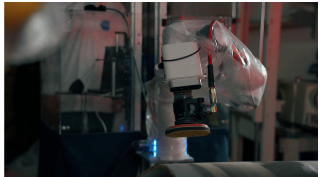
Figure 1: In this paper, we describe the development of a human-robot teaming solution for variable industrial sanding tasks that combines the strengths of the operator and robot through end-user programming and shared autonomy.
