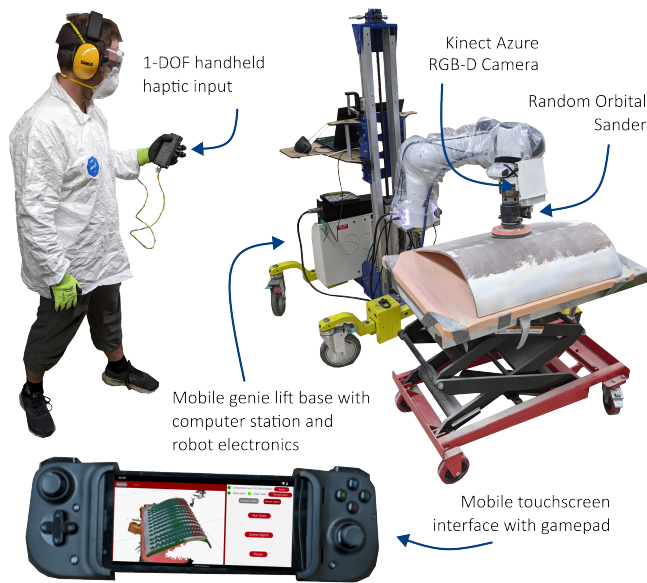
Figure 3: Overview of implementation. The worker’s interface uses a touchscreen gamepad and (optional) low degree-of-freedom haptic device to interact with the robot. The robot has a custom stand and end effector for sanding.
