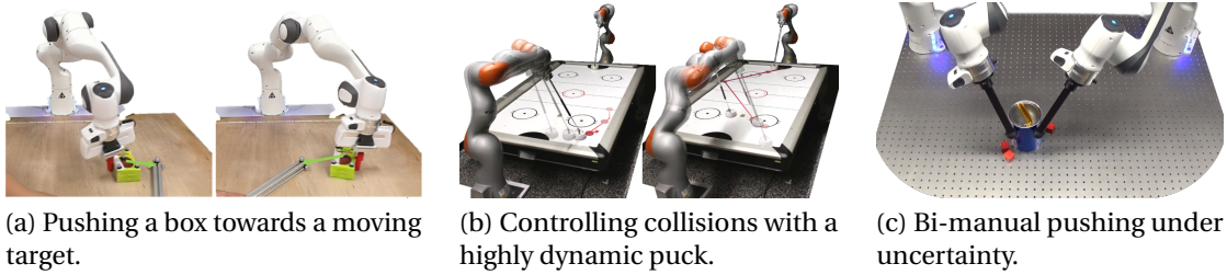
Figure 1.3: A selection of experiments on contact-rich manipulation conducted in the context of this thesis.
