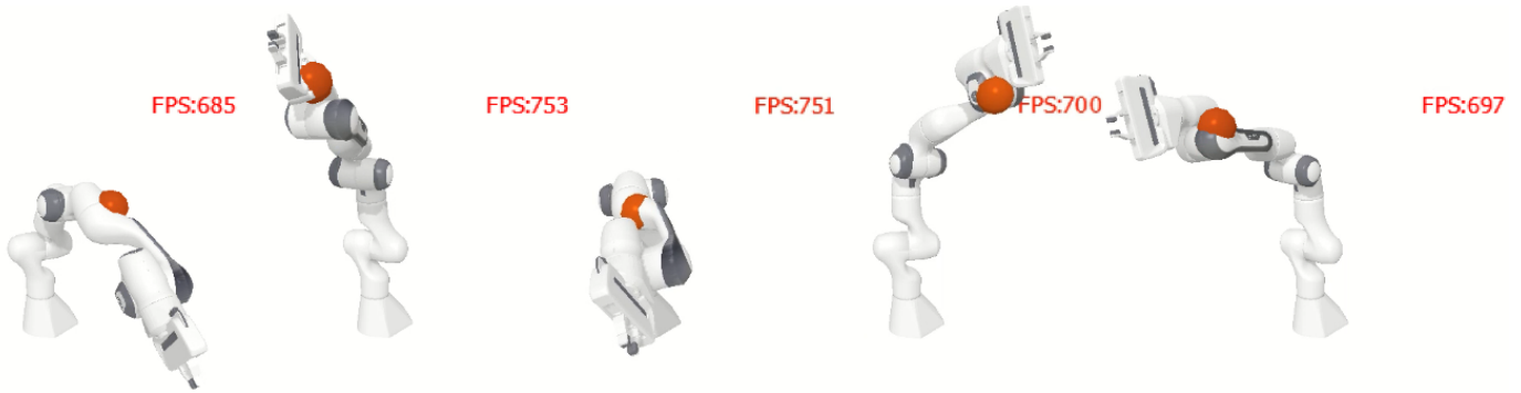
Fig. 4: Gradient projection for whole-body inverse kinematics using neural CDF. The centers of the red spheres are target points, where the radius of spheres is set to 0.05m .
