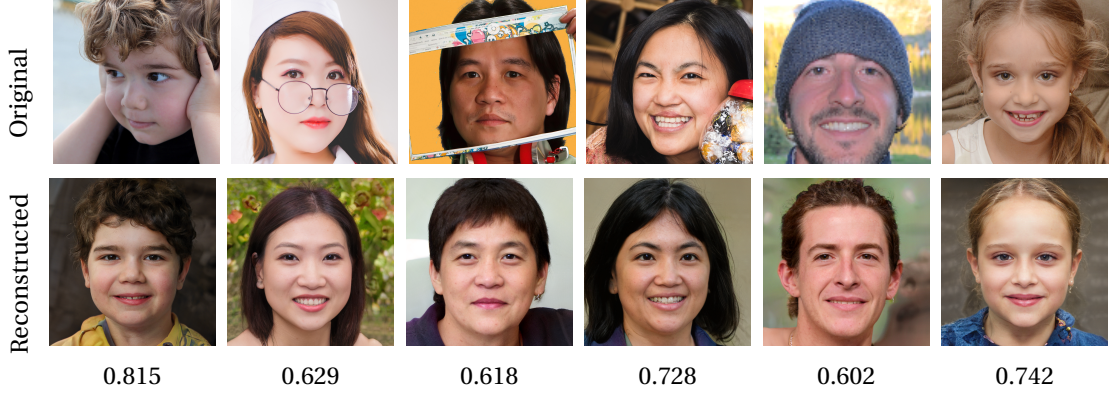
Figure 3.12: Sample face images from the FFHQ dataset and their corresponding reconstructed images using our template inversion method from ArcFace templates (used in a face recognition system). The values below each image show the cosine similarity between the corresponding templates of original and reconstructed face images.
