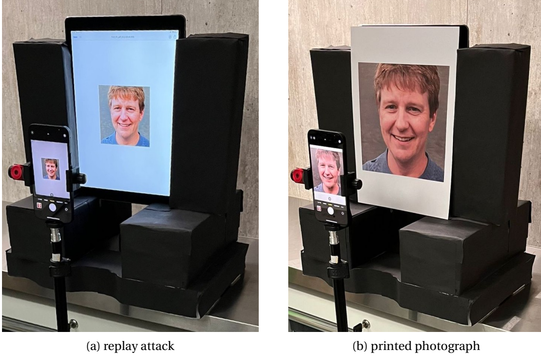
Figure 3.26: Our evaluation setup for performing different types of presentation and capturing presentation using mobile devices (a) replay attack using Apple iPad Pro, and (b) presentation attack using printed photograph
