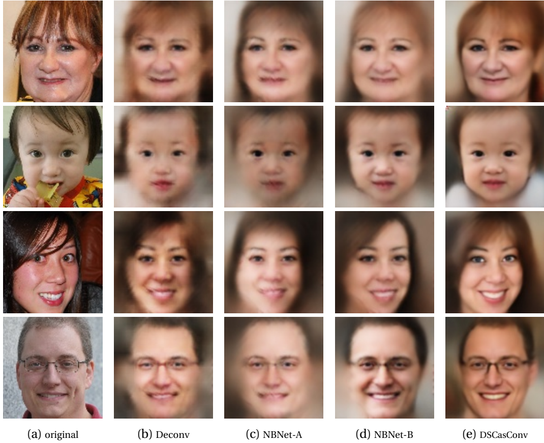
Figure 3.8: Sample face images from the FFHQ dataset and their reconstructed images from iResNet100-ArcFace templates using face reconstruction networks based on different blocks: (a) original image, (b) deconvolution, (c) NBNet-A, (d) NBNet-B, and (e) DSCasConv.
