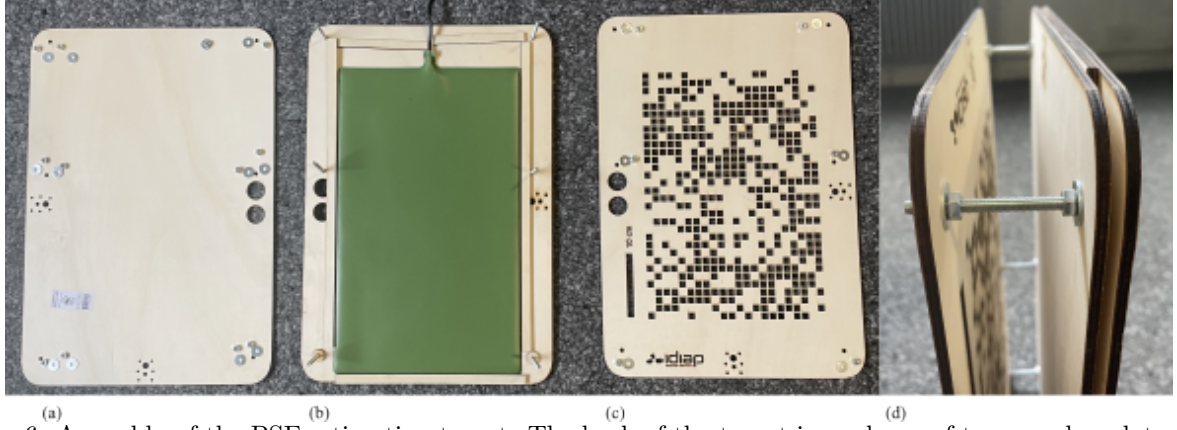
Figure 6: Assembly of the PSF estimation target. The back of the target is made up of two wooden plates with a heating plate between them: (a) middle heating cover panel (b) back panel and heater. The front panel (c) has 1cm-squares cut out according to a binomial distribution pattern. (d) in the assembled target, the pattern is 6cm away from the heating cover panel.
